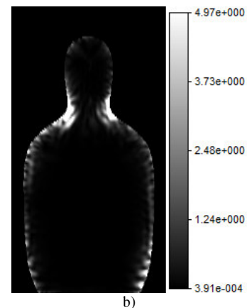
Figure 7. Near field distribution in the car (a) and SAR distribution inside of human body (b) at 1800 MHz frequency (source is base station antenna).
